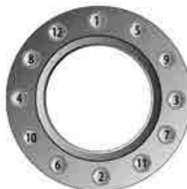
Fig 34 - 12 Bolt sequence
